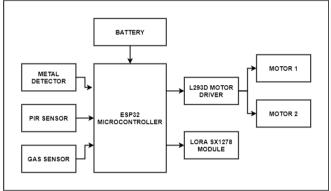
Fig -1: Block Diagram of Robot
