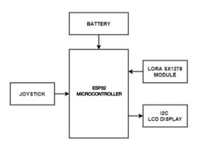
Fig -2: Block Diagram of Remote-control
